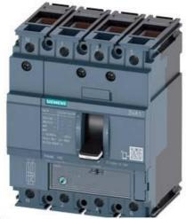
CIRCUIT BREAKER 3VA1 IEC FRAME 160 BREAKING CAPACITY CLASS S ICU=36KA @ 415 V 4-POLE, LINE PROTECTION TM220, ATFM, IN=80A OVERLOAD PROTECTION IR=56A ...80A SHORT CIRCUIT PROTECTION II=10 X IN NEUTRAL UNPROTECTED CABLE CONNECTION
